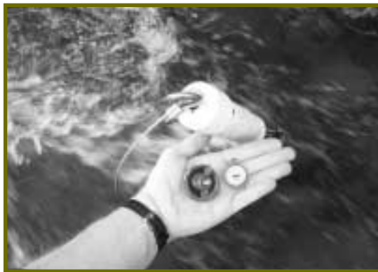
Onset's StowAway TidbiT temperature data logger fits securely into a housing anchored to the river bottom, where it collects a temperature reading every 15 minutes.
