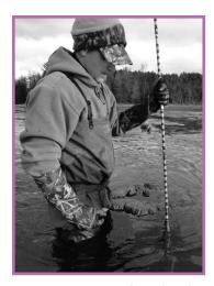
A sturdy rod marked with measured increments is a simple, useful tool for monitoring sediment depths.
