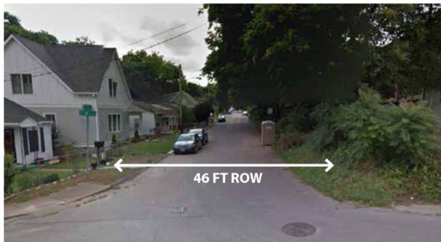
This block has a 46 foot Right of Way, the minimum width for installing green features and maintaining standard drive lanes.
