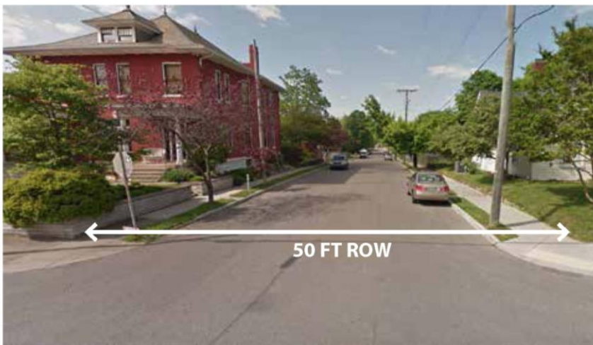
This block has a 50 foot Right of Way, letting us reduced drive lanes to create room for stormwater features
